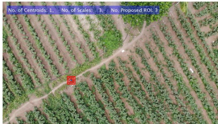
Fig. 5. A person in blue clothes is captured in the proposed regions (3 scales of red bounding boxes) while other objects are ignored.
